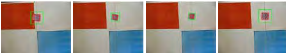
Figure 5. Bhattacharyya resizing. A simple red and blue checkered object is tracked across red, white and blue background regions by the ABCshift tracker, augmented with Bhattacharyya resizing. Frames 180, 200, 205, 206 shown. Due to rapid, jerky motion from frames 180 to 205, the search window has shrunk until it falls within the object region, risking relearning that background looks like object. ABCshift has detected this instability using the Bhattacharyya metric, and automatically corrects the estimated object region and search window size in frame 206. Green and red squares indicate the search window and estimated object size respectively. This movie, PeopleTracking1ABCshift.avi , can be viewed at the project website (see references).
