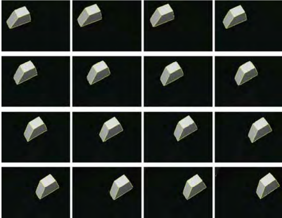
Figure 3. Tracking simple shape in a structured environment. The modelbased polyhedral object pose estimation is used to compute the camera displacements during the image sequence
