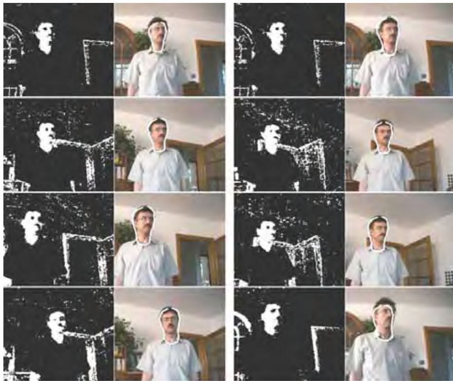
Fig. 4. ASM-based face tracking, using gradient. Frames #1, #2, #20, #60, #80, #100, #120.
