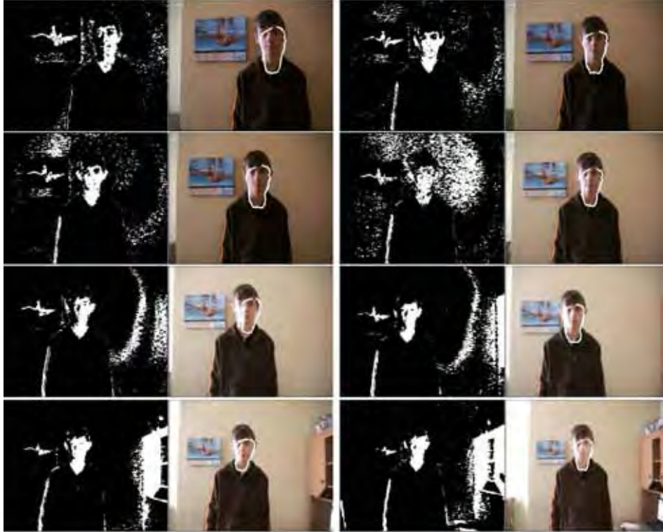
Fig. 12. ASM-based face tracking in varying illumination using intensity gradient and phase of Gabor filter responses. Frames #1, #50, #55, #56, #60, #70, #100 and #200.
