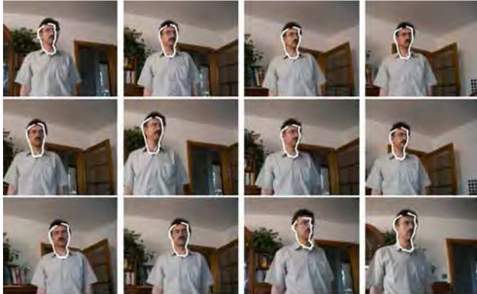
Fig. 10. ASM-based face tracking using distance to the edge of the face mask, intensity gradient and coherence of the phase. The number of modes is set to four. Each 10-th frame of 120 frames long sequence is presented.
