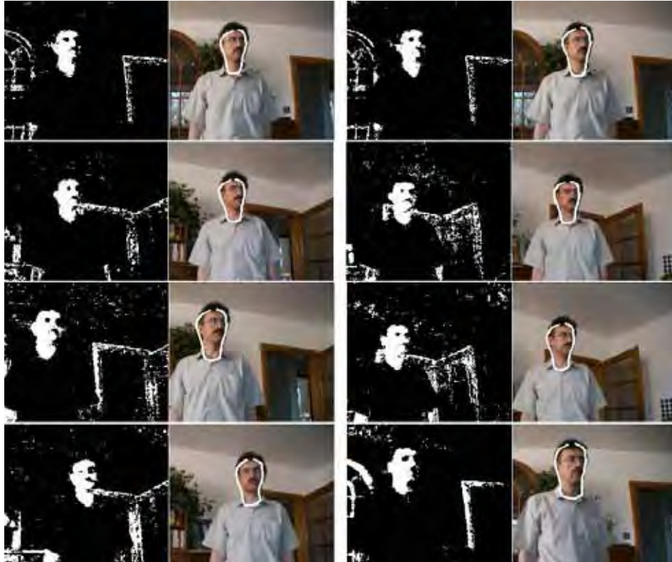
Fig. 9. ASM-based face tracking using the distance to the edge of face mask, intensity gradient and coherence of the phase. Frames #1, #2, #20, #40, #60, #80, #100 and #120.
