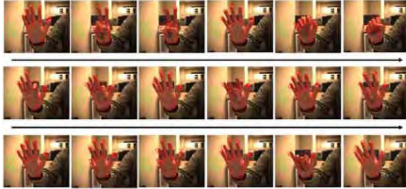
Figure 15. Demonstration of finger tracking with 200 particles. The projection of OpenGL hand model's edge is drawn on images.
