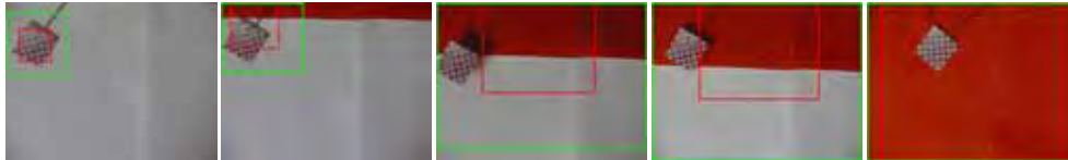
Figure 1. A simple blue and red chequered object, moving from a region of white background into a region of red background. CAMSHIFT fails as soon as the object moves against a background with which it shares a common colour. Frames 350, 360, 380, 400, and 450 shown. Green and red squares indicate the search window and estimated object size respectively. This movie, RedWhite1CAMSHIFT.avi, can be viewed at the project website (see references).
