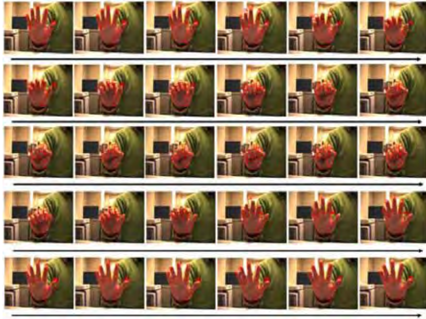
Figure 13. Five-finger tracking with 50 particles by our method. The projection of OpenGL hand model's edge is drawn on the images
