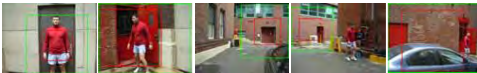
Figure 3. Person tracking with CAMSHIFT from a moving camera in a cluttered, outdoors environment. Frames 1, 176, 735, 1631 and 1862 shown. Since the tracked person wears a red shirt, CAMSHIFT tends to fixate on red regions of background, including brick walls and doors, and repeatedly loses the tracked person. Green and red squares indicate the search window and estimated object size respectively. This movie, PeopleTracking1CAMSHIFT.avi can be viewed at the project website (see references).
