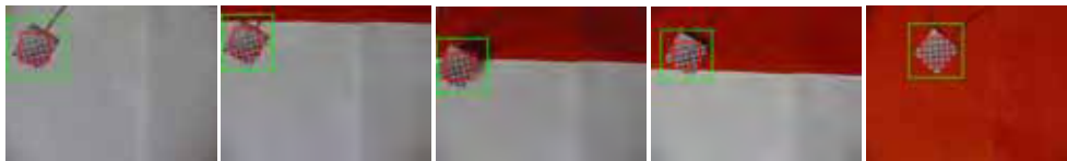
Figure 2. ABCshift tracks successfully. Frames 350, 360, 380, 400, and 450 shown. Green and red squares indicate the search window and estimated object size respectively. This movie, RedWhite1ABCshift.avi, can be viewed at the project website (see references).
